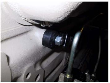
Look, here a sample how the sensors are mounted on an NTA 855 Cummins
